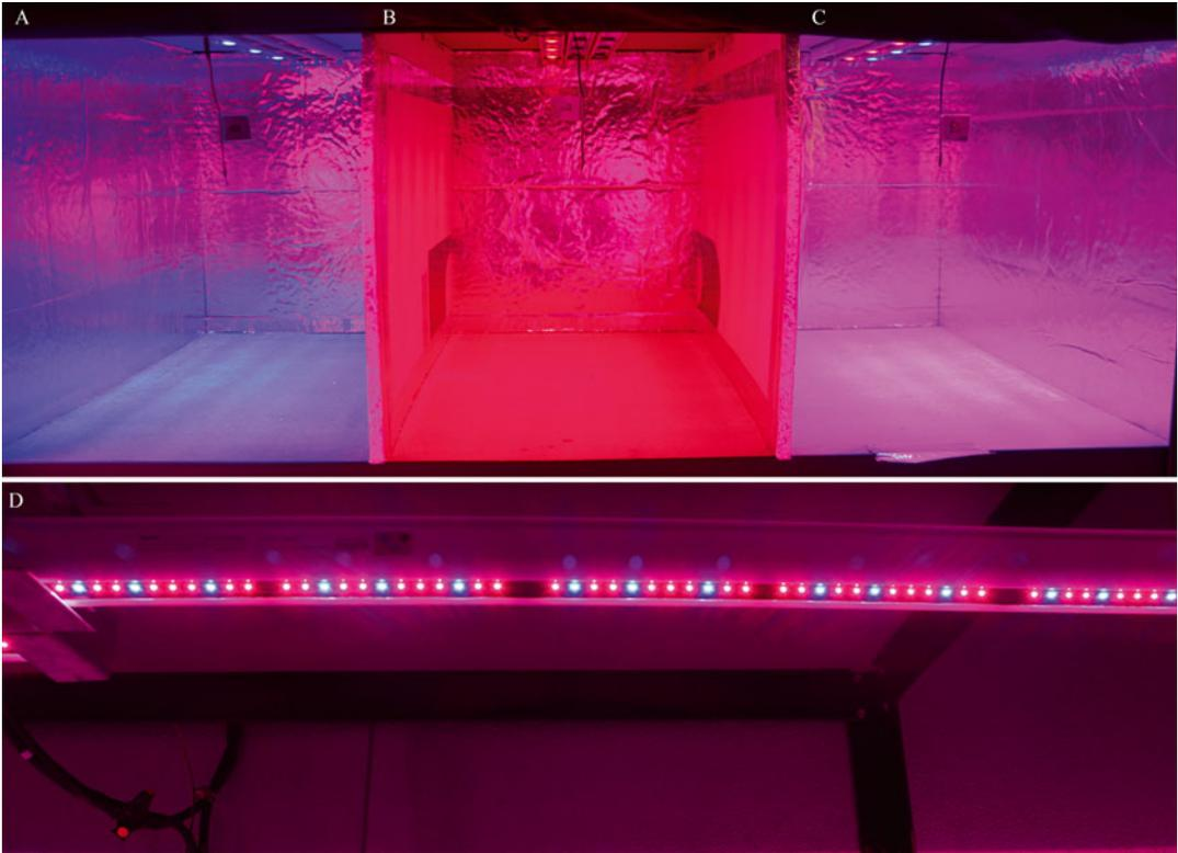
**Fig. 2** Light emitting diodes in controlled environment room providing desired light qualities for culturing *Veratrum californicum* plantlets. 20  $\mu\text{mol}/\text{m}^2/\text{s}$  monochromatic blue (a), 20  $\mu\text{mol}/\text{m}^2/\text{s}$  red (b), 20  $\mu\text{mol}/\text{m}^2/\text{s}$  red–blue (c), and 40  $\mu\text{mol}/\text{m}^2/\text{s}$  red–blue (d)
