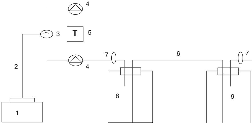
**Fig. 1** Diagram of the temporary immersion system showing the different components: (1) Air compressor; (2) reinforced PVC tubing (ID 10 mm); (3) pressure regulation station; (4) three-way solenoid electrovalve; (5) programmable timer; (6) autoclavable silicone tubing (ID 6 mm); (7) sterilizable filter (0.22  $\mu\text{m}$ , Midisart 2000, Sartorius AG); (8) culture flask; (9) medium reservoir vessel
